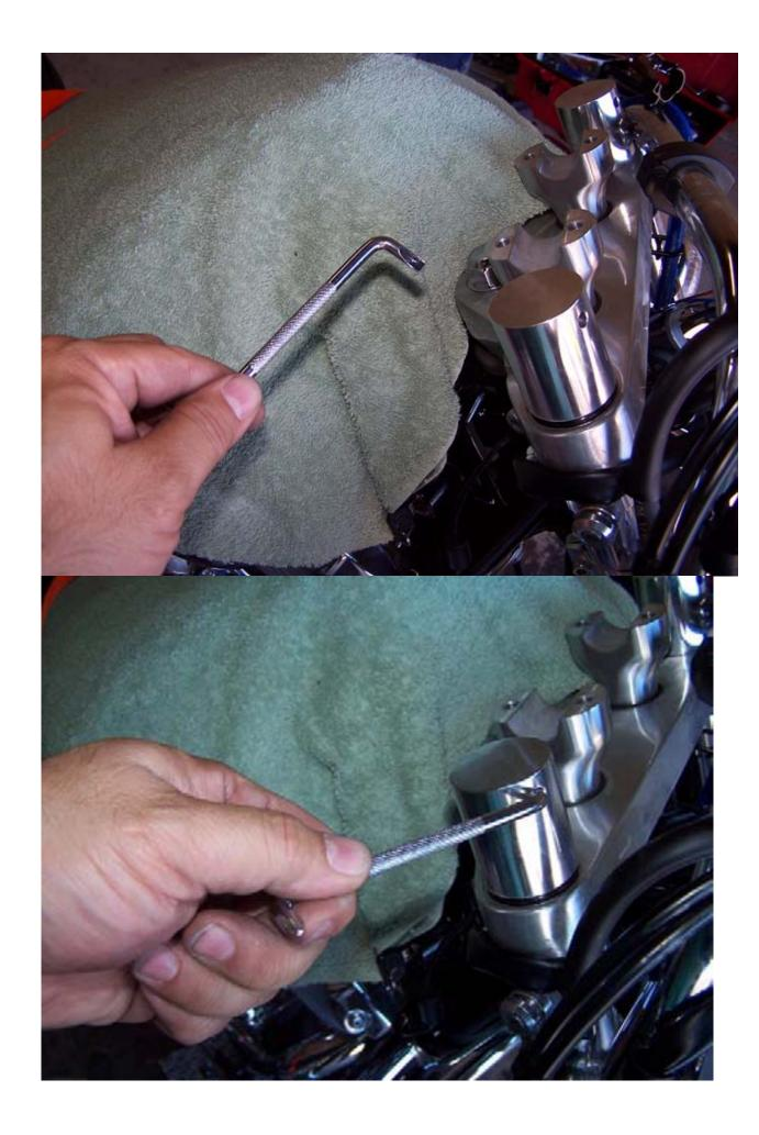
Once both sides are installed, you have to loosen the clamps on the triple tree and slide the forks down. On my Custom, there were five things I had to loosen per side. The top and bottom clamps, the Turn Signal bracket (two screws) and the two clamps for my Memphis Fats windshield. Here are shots of the top, bottom and Turn Signal clamps.
